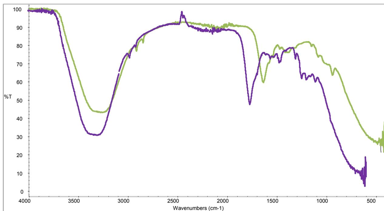
Figure 4.6 FTIR spectra of Chitosan from Sample A and sample B
